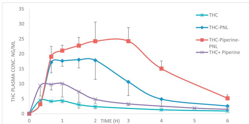
Fig. 5. Plasma THC concentration vs. time plot (mean ± SEM) following PO administration of THC, THC-PNL, THC-Piperine-PNL and THC with piperine in solution. THC dose 20 mg/kg, piperine dose 10 mg/kg (n = 6 for each group).
