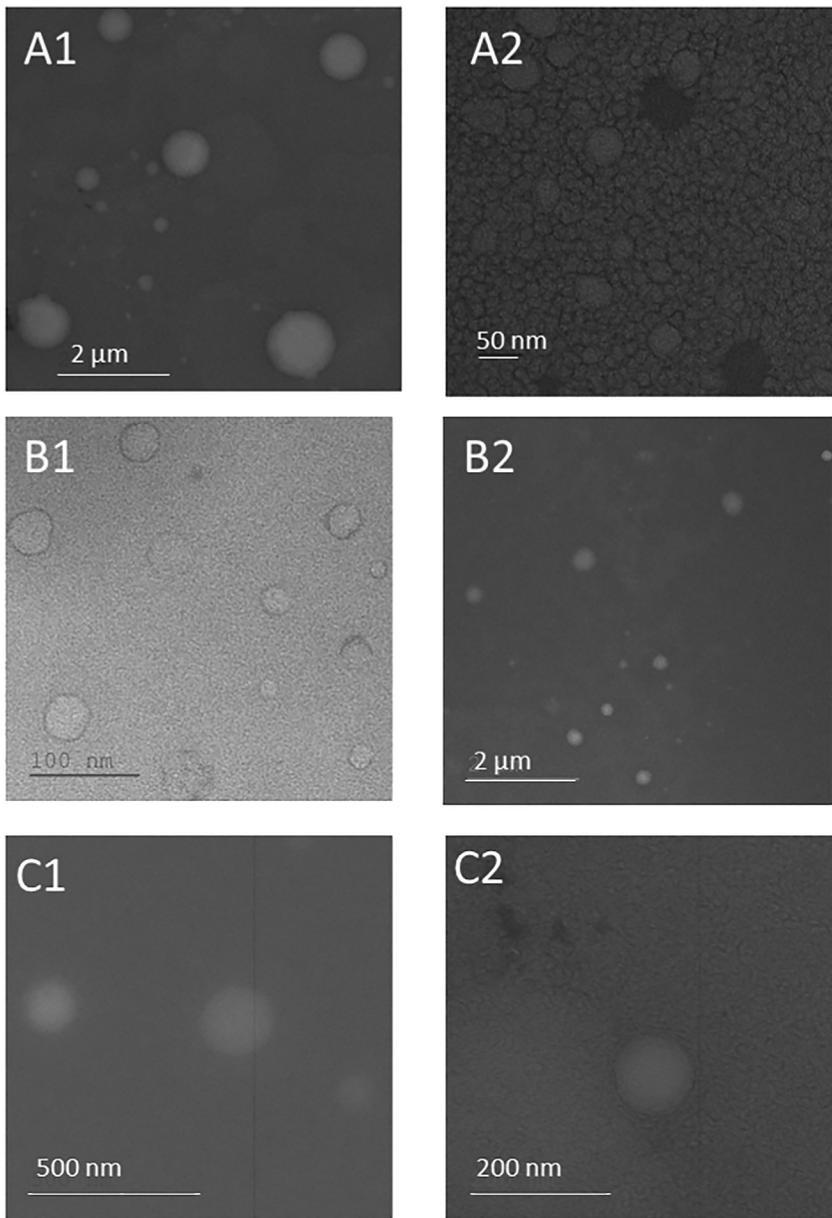
Fig. 1. TEM analysis of PNL dispersion: blank PNL A1 (1:10 v/v) and A2 (1:50 v/v), CBD-piperine-PNL B1 (1:10 v/v) and B2 (1:50 v/v), THC-piperine-PNL (1:10 v/v) and (1:50 v/v)
